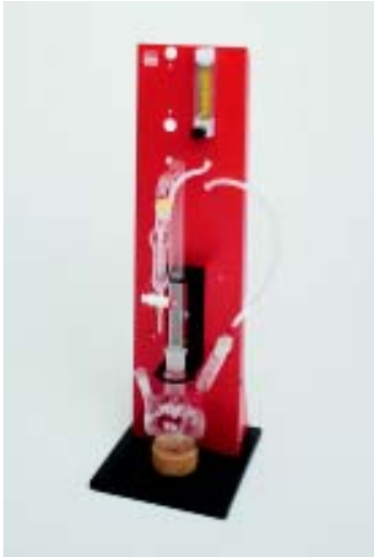
KLFC: Readily liberated cyanide, single sample apparatus
